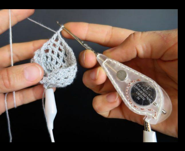
This crochet hook translates electrical resistance into vibration, making electrical resistance a tangible property of an E-Textile making process. The Ohm Hook allows you to develop an electrical sense for the materials you work with. For example, if you are crocheting stainless steel yarn to make a stretch sensor you can tailor your design to the range of resistance you want because you immediate feedback on the resistance of what you are making.
