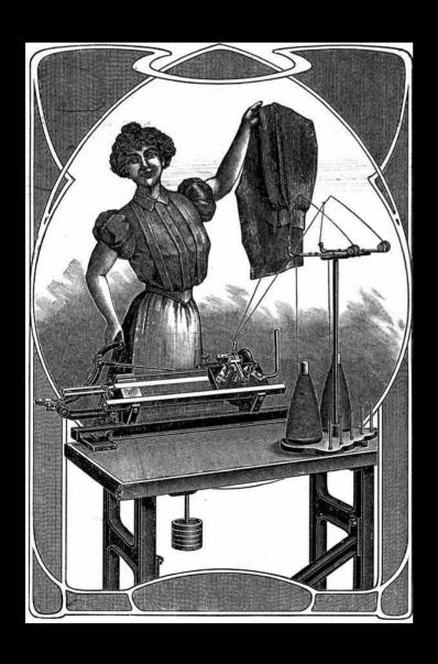
The first simple hand-powered flat-bed knitting Machines were constructed for home use by the cottage industry in 1890.
